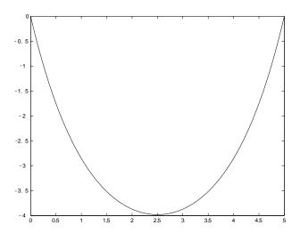
**Figure 1.14.** *Hanging cable with uniformly distributed mass.*
