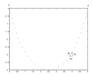
**Figure 1.15.** *Discretized hanging cable with uniformly distributed mass.*
