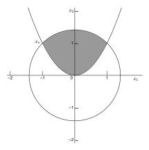
**Figure 1.2.** *Nonlinear optimization problem with inequality constraints.*
