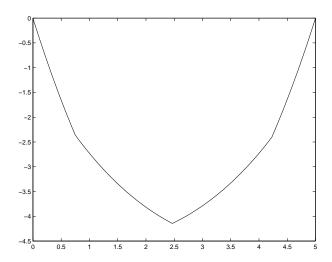
**Figure 1.18.** Hanging cable with a nonuniform mass distribution.
